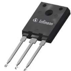
Fully isolated package TO-247
