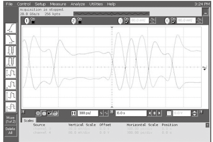
Data Waveforms, 2.5Gbps (left) & 5.0Gbps (right)
