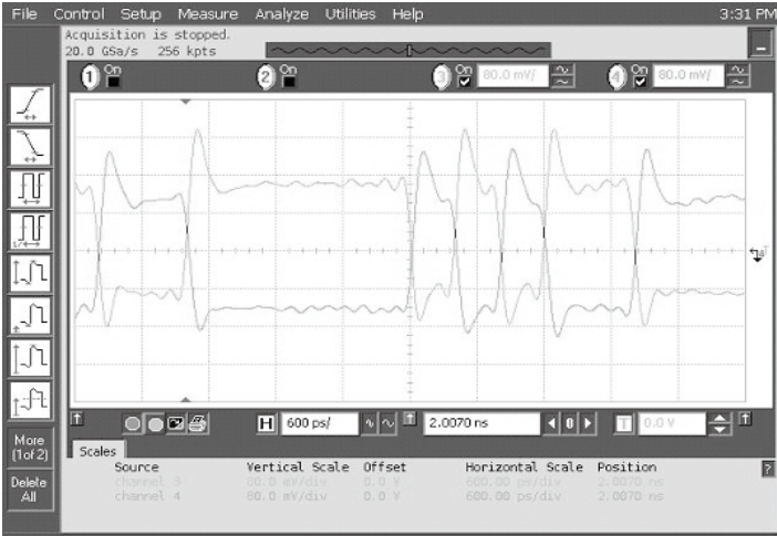
Data Waveforms, 2.5Gbps (left) & 5.0Gbps (right)
