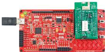
Fig 4: Programming and debugging with CY8CKIT-042-BLE BLE Pioneer Kit Baseboard
