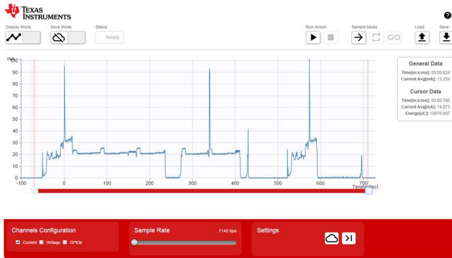
Figure 12. Wireless Scope Measurement of Sample CC3100 Program Initialization
