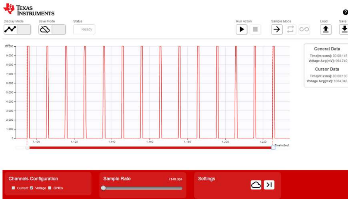
Figure 20. Wireless Scope Measurement of 100 Hz 1-ms pulses
