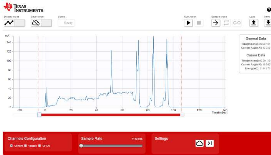
Figure 10. Wireless Scope Measurement of Transceiver Mode
