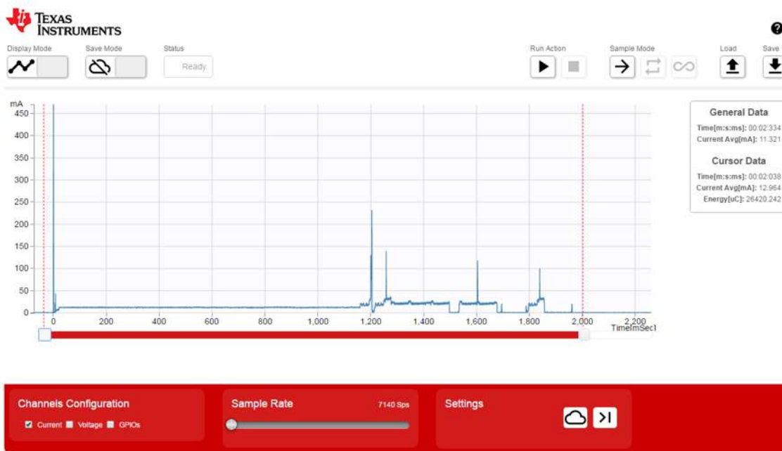
Figure 14. Wireless Scope Measurement of CC3100 Wake-Up From Shutdown
