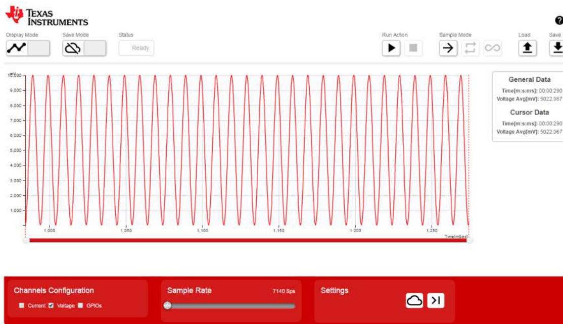
Figure 18. Wireless Scope Measurement of 100-Hz Sine Wave
