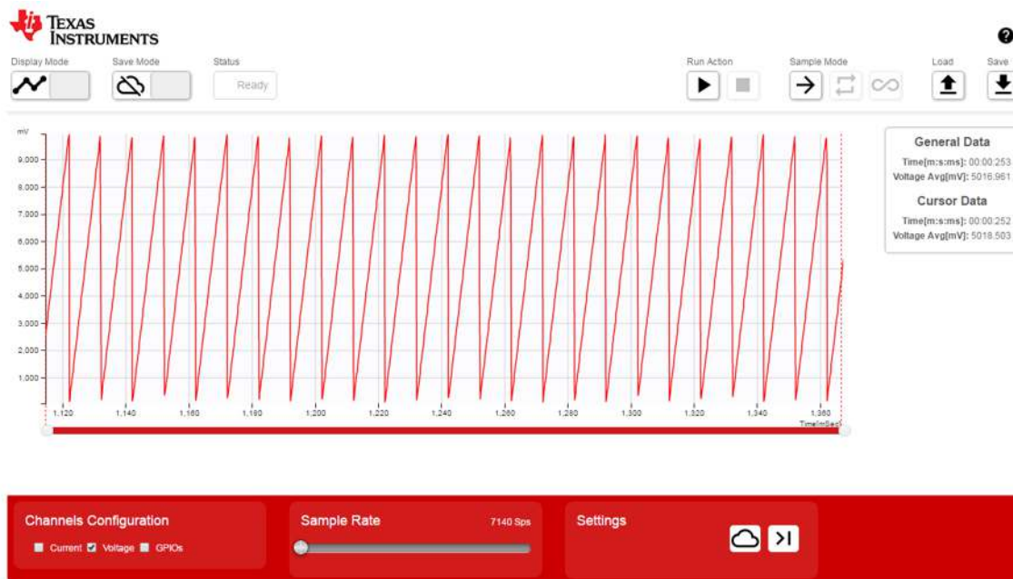
Figure 22. Wireless Scope Measurement of 100-Hz Ramp Wave
