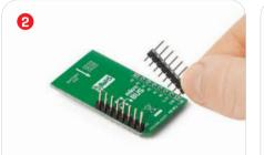
Turn the board upside down so that the bottom side is facing you upwards. Place shorter pins of the header into the appropriate soldering pads.
