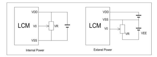
VDD-V0: LCD Driving Voltage VR: 10k-20k
