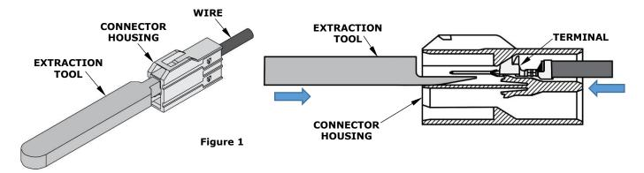
4. Push the extraction tool into the connector housing until the blade stops on the locking tab inside the housing. See Figure 2.
