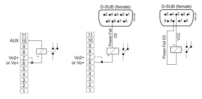
Fig. 19 Option D2: Examples of relay control to monitor a power failure.
