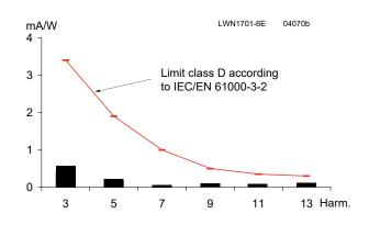
Harmonic currents at input current, measured at V<sub>1</sub> = 230 VAC,  $I_{o} = I_{o \text{ nom}} (LWN1701-6E).$
