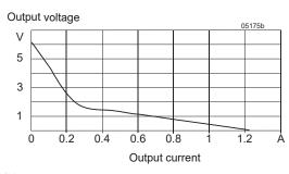
Fig. 21 Output voltage versus output current, while the shutdown is activated  $(V_i = V_{i \text{ nom}})$ .
