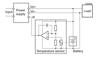
Schematic circuit diagram of a system with battery backup and temperature-controlled charging.
