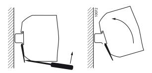
Fig. 16a Snap-fit mounting to DIN-Rail.
