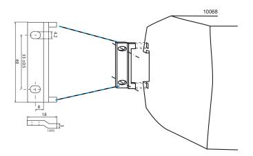
Fig. 23 Wall mounting with mounting brackets HZZ00618-G
