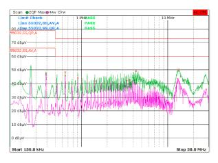
Fig. 11a Conducted emissions of LW models with feature E: Disturbances at the phase input according to EN 55032, measured at  $V_{\rm inom}$  and  $I_{\rm onom}$ . (LWN1701-6EG)
