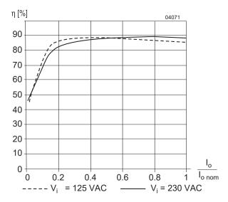
Fig. 3 Efficiency versus load (LWN 2660-6)
