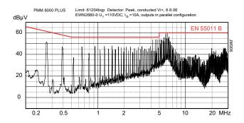
Fig. 12a Conducted emissions of EW models: Disturbances (peak) at the phase input according to EN 55011, measured at  $V_{\rm i \, nom}$  and  $I_{\rm o \, nom}$ . (EWN2660-0)
