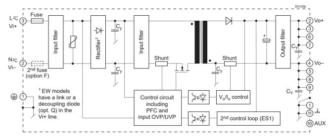
Fig. 1 Single-output converters (125 W).
