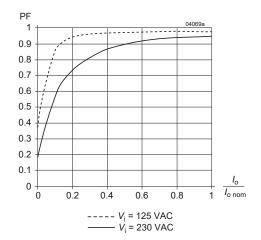
Fig. 5 Power factor versus load (LWN2660-6)
