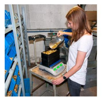
PCE-PCS 30 is a tabletop scale or balance with accurate weighing and piece or part counting functions. Ideal for use in laboratory, office, inventory and miscellaneous industrial applications, this portable scale can be powered by battery or by the included electric power supply. The scale's built-in RS-232 port enables data transfer and printing.
