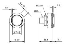
DC 24V (8.4 ... 32V) Max. 200 mA Adjustable PNP/NPN; NO/NC Adjustable Protection of all cables/lines Protected against short circuit and overload Max. 5V at 200 mA load current Max. 40 mA -30°C ... +65°C Front side IP69K maximum unevenness in mounting surface < 0.1 mm IK08 IO-Link specification V1.1 on 80 %  $U_v$ +, off 0 ... 20 %  $U_v$ + Capacitive Touch
