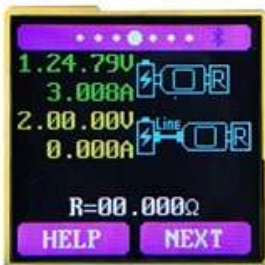
Data Connection Cable Impedance Measurement Interface
