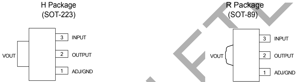
Figure 2. Pin Configuration of AZ1117B (Top View)
