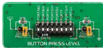
Figure 6-5: Button press level DIP switch (tri-state)
