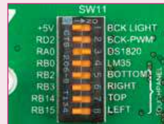
Figure 20-3: Enabled SW11.3 DIP switch
