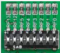
Figure 6-2: Tri-state DIP switch on PORTF
