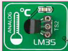
Figure 21-2: LM35 correctly placed in socket
