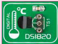
Figure 20-2: DS1820 correctly placed in socket
