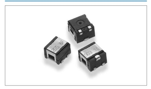
TE Connectivity (TE) are pleased to introduce this tiny (4mm square) multiturn trimmer potentiometer. The 3240 Series is designed with a footprint meeting EIA and other international board layout standards. It is also compatible with all surface mount manufacturing processes. It is ideally suited to small sensors where its 10 turn setability and small size enables it to stand out from most other competitors.
