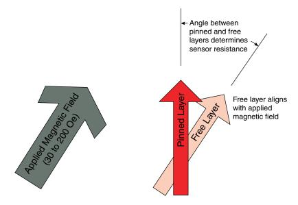
The sensor element free layers will align with the external field. As the applied field changes direction, the angle between the free layer and the pinned layer changes, changing the resistance of spintronic Tunneling Magnetoresistance (TMR) elements, which changes the device output voltages.
