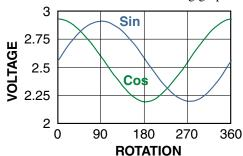
The output is insensitive to magnet spacing over a wide range. Signal is lost if the magnet is too far away; if the magnet is too close the outputs will be non-sinusoidal. A relatively large magnet-sensor airgap is possible with the magnet provided with the kit, although smaller magnets will require a smaller gap.
