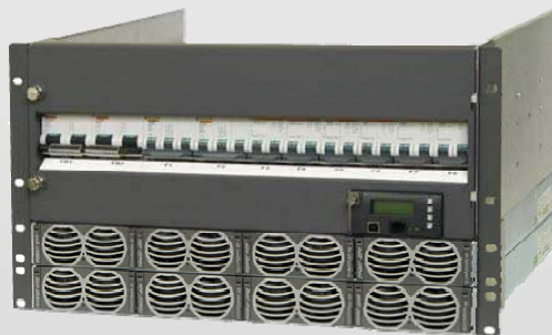
19", 6 RU Dual Voltage System (-48 VDC / 12.5 kW & +24 VDC / 4.5 kW) with Controller, Load & Battery Distribution
