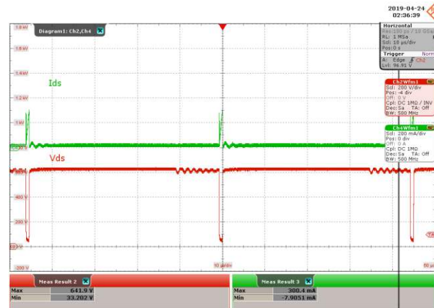
Figure 15 – Drain Voltage and Current Waveforms. 440 VAC, 120 mA Output. Upper: I_{DRAIN} , 200 mA / div. Lower: V_{DRAIN} , 200 V, 10 \mu s / div. I_{MAX} = 300.4 mA, V_{MAX} = 641.9 V.
