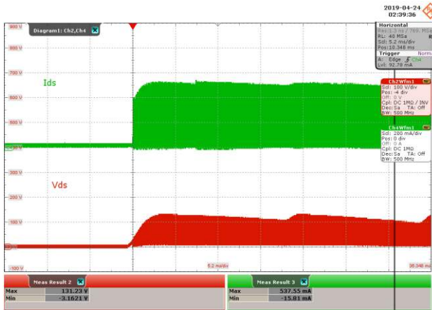
Figure 16 – Drain Voltage and Current Waveforms. 85 VAC, 120 mA Output. Upper: I_{DRAIN} , 200 mA / div. Lower: V_{DRAIN} , 100 V, 5.2 ms / div. I_{MAX} = 537.55 \text{ mA} , V_{MAX} = 131.23 \text{ V}
