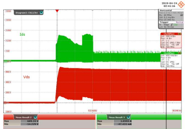
Figure 17 – Drain Voltage and Current Waveforms. 440 VAC, 120 mA Output. Upper: I_{DRAIN} , 400 mA / div. Lower: V_{DRAIN} , 200 V, 5.2 ms / div. I_{MAX} = 1.0593 \text{ A} , V_{MAX} = 689.3 \text{ V}
