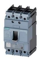
circuit breaker 3VA5 UL frame 125 breaking capacity class H 65kA @ 480 V 3-pole, line protection TM230, FTAM, In=25A overload protection Ir=25A fixed short-circuit protection Ii=6...12 x In UL489 SB (naval), 50 deg. cel. cable connection on both sides
