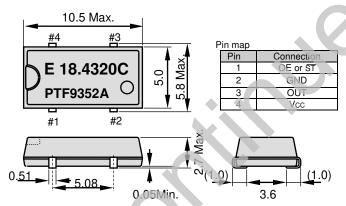
The metal case inside of the molding compound may be exposed on the top or bottom of this product. This purely cosmetic and does not have any effect on quality, reliability or electrical specs. Note.
