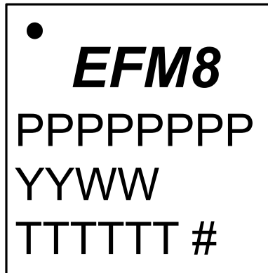
Figure 7.3. QFN32 Package Marking
