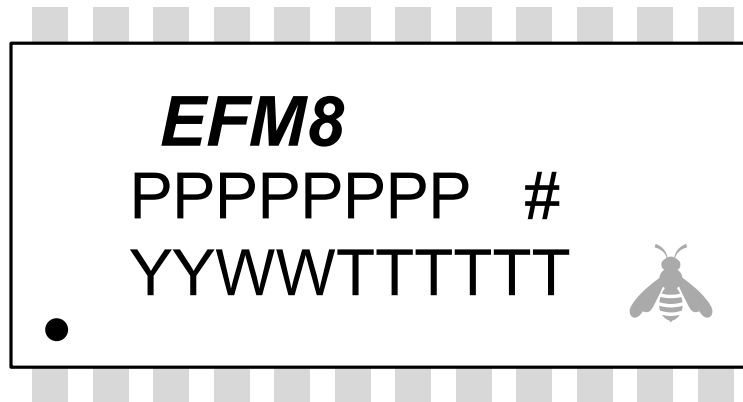
Figure 10.3. QSOP24 Package Marking
