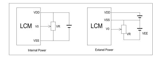
$V_{DD^{\sim}}V_0$ : LCD Driving voltage
