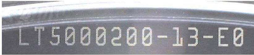
Figure 3-2. Wafer Identification Code 1
