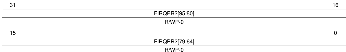
Figure 15-19. FIQ/IRQ Program Control Register 2 (FIRQPR2) [offset = 18h]
