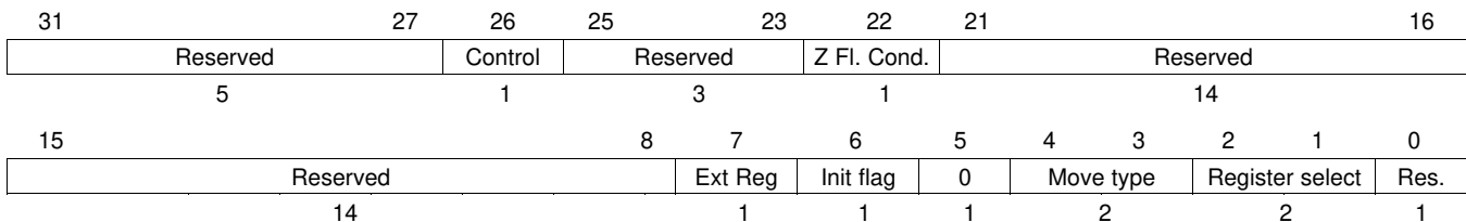
Figure 20-154. MOV32 Control Field (C31:C0)
