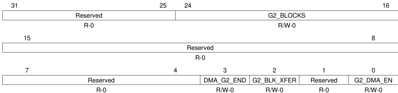
Figure 19-42. ADC Group2 DMA Control Register (ADG2DMACR) [offset = 54h]
