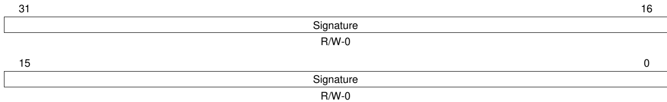
Figure 32-6. EFC Self Test Cycles Register (EFCSTSIG) [offset = 4Ch]
