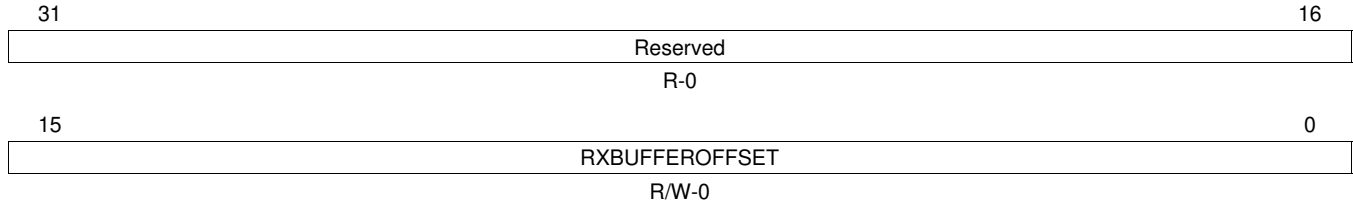
Figure 28-66. Receive Buffer Offset Register (RXBUFFEROFFSET)
