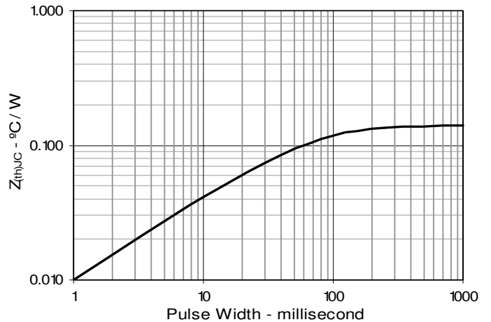
Fig. 12. Maximum Transient Thermal Impedance
