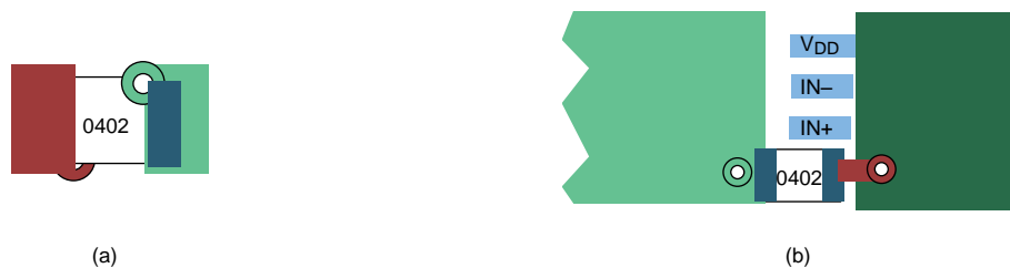
Figure 21. Typical Decoupling Capacitor Layouts
