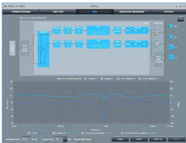
Figure 11.17: MA2304DNS GUI used for configuring the DSP
