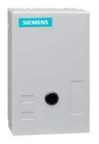
Non-reversing NEMA contactor, Size 1, Three phase full voltage, Contactor amp rating 27A, 3 wire (NO aux included), 110V 50Hz / 120V 60Hz coil, Non-combination type, Enclosure NEMA type 1, Indoor general purpose use, Standard width enclosure
