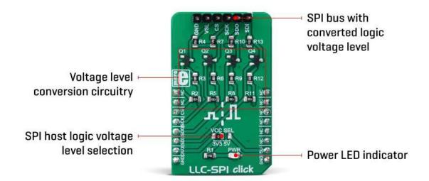
The SPI protocol was first introduced by Motorola, in the '80s. The circuit is divided into low-side and high-side sections for future reference, however, both up-shifting, and down-shifting of the voltage level is possible. The mechanisms are slightly different, so each will be explained separately.
