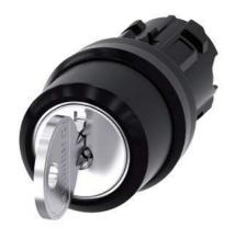
RONIS key-operated switch, 22 mm, round, plastic, lock number SB30, with 2 keys, 3 switch positions I-O<II, left latching, right momentary contact type, actuating angle 2x45°, 10:30h/12h/13:30h, key removal I, possible special locks: SB31, 421, 455, with laser labeling, upper case and lower case, always upper case at the beginning of the word
