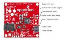
The charge current is set by resistor R1 in the schematic. By default it comes set to a maximum charge current of 450mA. It's recommended that batteries not be charged at greater than their capacity rating; thus, the smallest battery that should be charged with the Sunny Buddy is 450mAh.
