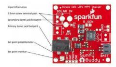
There are also additional footprints for attaching 3.5mm screw terminals or an additional barrel jack to the board. Please note that if you intend to use two solar panels, you **must** clear solder jumper JP1 (it ships closed by default) and close solder jumper JP2 (it ships open by default). Failure to do
