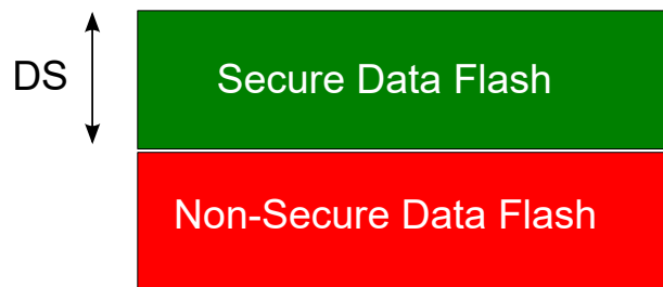
Figure 13-3. SAM L11 Data Flash Memory Mapping
