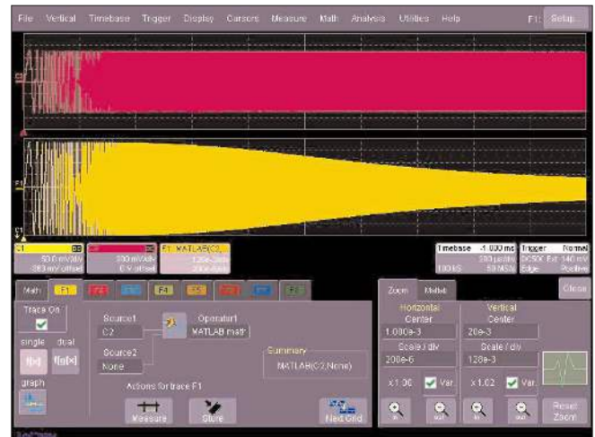
A user-created MATLAB low-pass filter is easily inserted as function F1 in the WaveMaster user interface.
