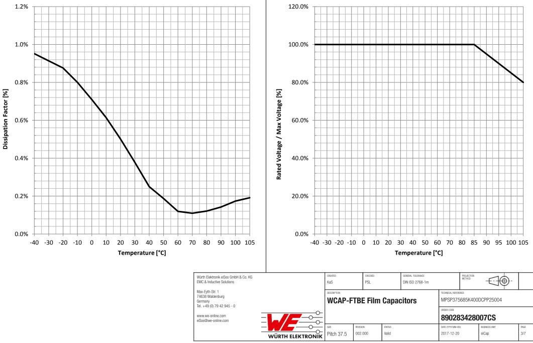
**Rated Voltage vs. Temperature:**
