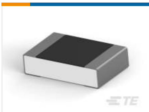
TE Part #1-2176382-8 RQ 0805 200K 0.1% 10PPM 5K RL
