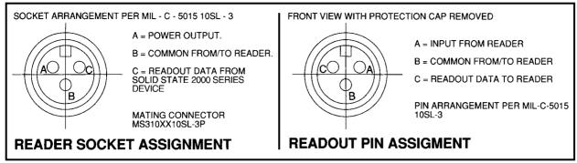
FOR MATING CONNECTOR TO OUTPUT PC MOUNT UNIT USE MS 3102A-10SL-3P
