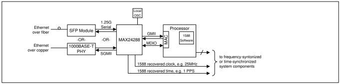
Example 2: Multiport System with Switch-Connected 1588 Slave Node
