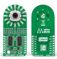
Rotary R click™ carries a **15-pulse incremental rotary encoder** with detents, surrounded by a **ring of 16 red LEDs**. It communicates with the target board through mikroBUS™ **SPI lines** (CS, SCK, MISO, MOSI), and three additional lines for outputting the Encoder info: ENCB OUT, ENCA OUT and SW (in place of the standard AN, RST and INT pins, respectively). Rotary R click™ can be used with either a 3.3V or 5V power supply.
