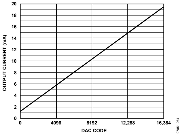
Figure 63. Gain Curve for FSC[9:0] = 512, DAC Offset = 1.228 mA
