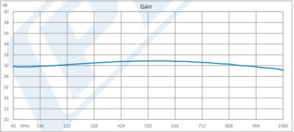
Click the following link (or enter part number in "SEARCH" on website) to obtain additional part information including price, inventory and certifications: 1.3 dB NF Low Noise Amplifier, Operating from 20 MHz to 1 GHz with 30 dB Gain, 18 dBm P1dB and SMA PE15A1051
