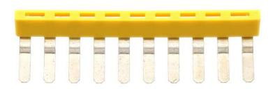
External insulated cross-connector, No. of poles: 10, Mounting type: Plug in, Width: 59.6 mm, Rated current: 27 A; Colour: Yellow
