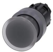
Illuminated mushroom pushbutton, 22 mm, round, plastic with metal front ring, clear, 30 mm, momentary contact type, with laser labeling, upper case and lower case, always upper case at the beginning of the word
