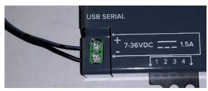
when connecting power to the E12, don't worry because the input is reverse polarity protected.
