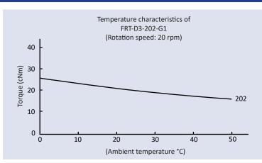
• **Temperature characteristics:** A rotary damper's torque varies according to the ambient temperature. In addition, as shown in the graph above, the torque decreases as the ambient temperature increases, and the torque increases as the ambient temperature decreases. This is because the viscosity of the silicone oil inside the damper varies according to the temperature. When the temperature returns to normal, the torque will return to normal as well.
