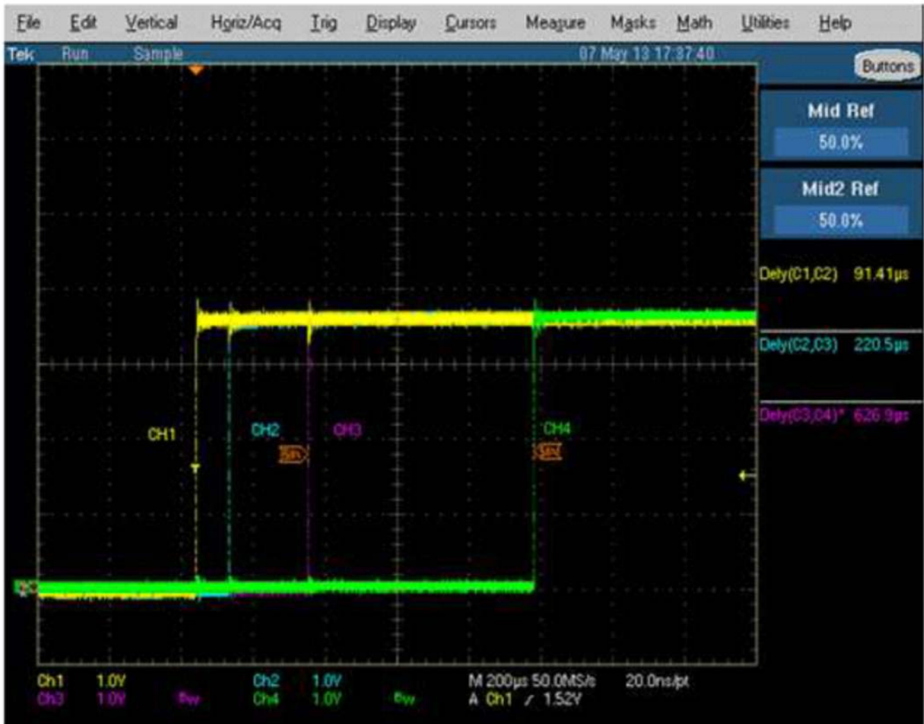
Figure 33. Programmable Turn on Delay Time
