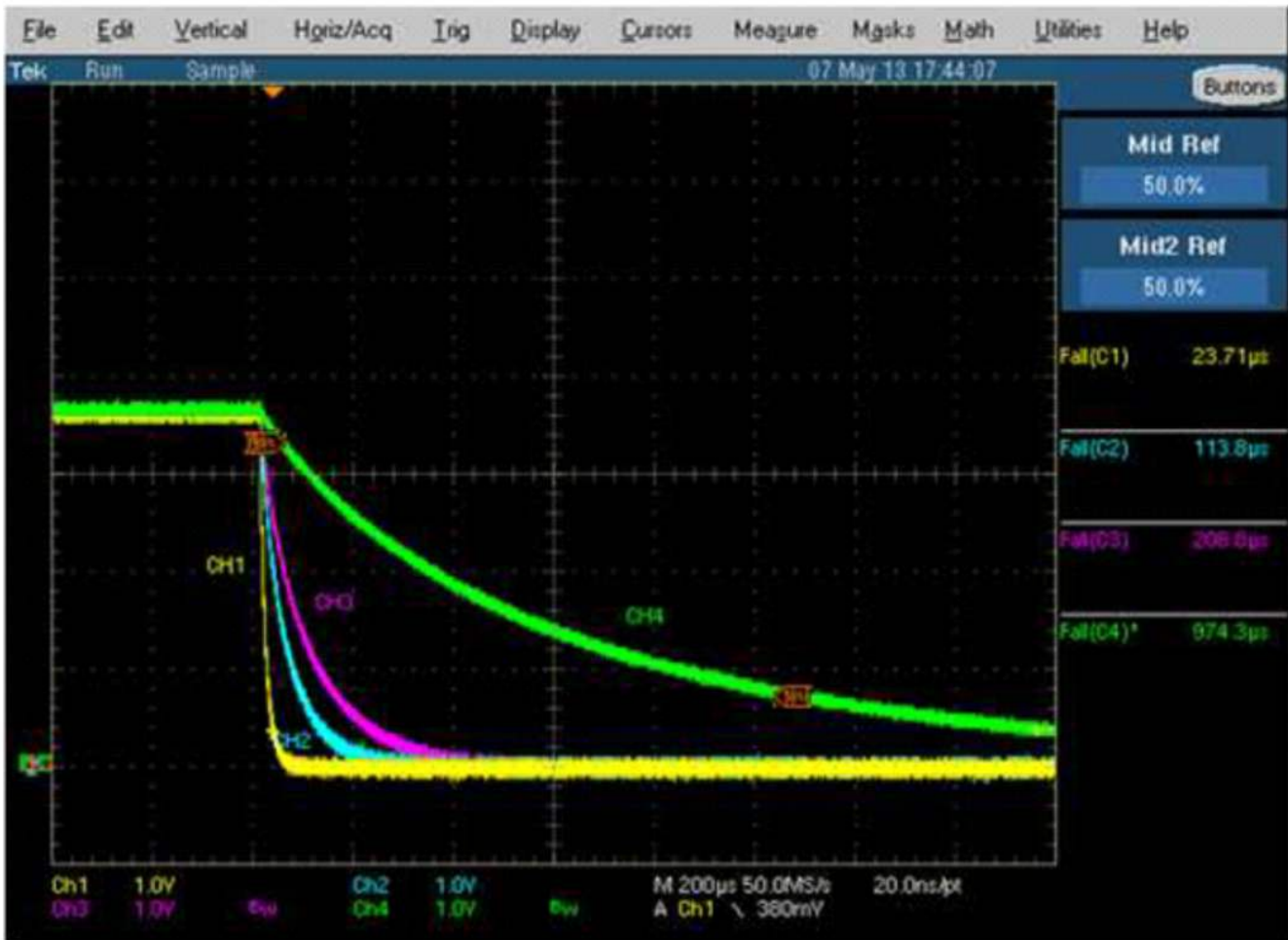
Figure 34. Programmable Output Discharge (Fall Time Control)
