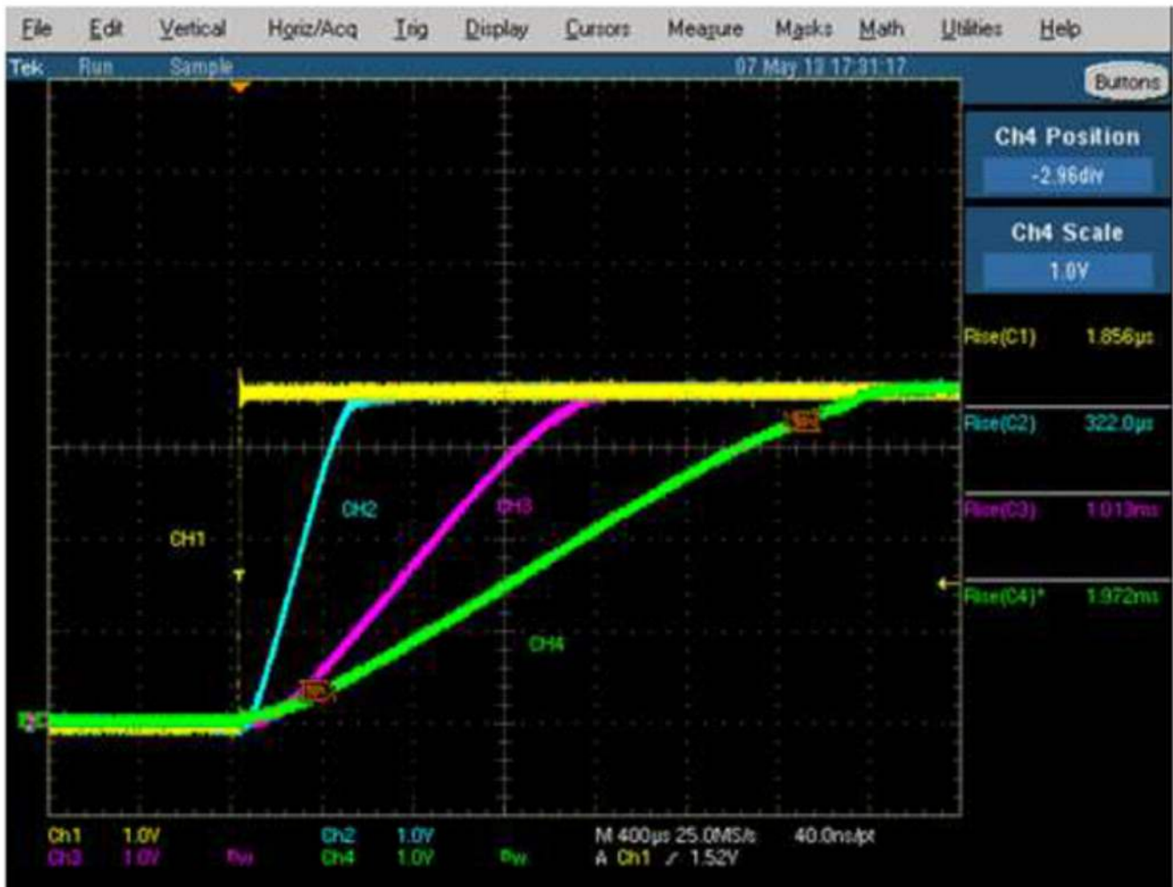
Figure 32. Programmable Slew Rate Control
