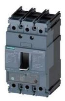
circuit breaker 3VA5 UL frame 125 breaking capacity class S 25kA @ 480 V 3-pole, line protection TM240, ATAM, In=100A overload protection Ir=80A ...100A short-circuit protection Ii=5...10 x In nut keeper kit on both sides
