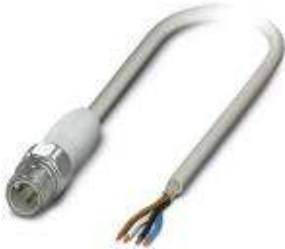
Sensor/Actuator cable, 4-position, PP-EPDM halogen-free, Gray RAL 7035, shielded, Plug straight M12, A-coded, on Free cable end, Cable length: 1.5 m, Hygienic design, With high-grade steel knurl
