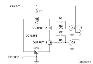
In conventional push-pull bipolar designs, forward base drive is controlled by R1-R3. Rapid turn-off times for the power devices are achieved with speed-up capacitors C, and C2.
