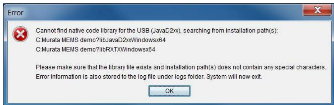
Figure 38. Error message when USB library is not found because of special characters
