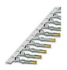
Crimp contact, Socket, rolled, Taped articles, number of pieces per reel: 10000, contact diameter: 1 mm, crimp range: 0.22 mm $^2$  ... 0.56 mm $^2$ , Item is lead-free in accordance with RoHS II without Exemption 6c (Pb <0.1%)
