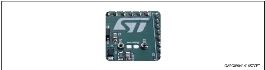
Figure 4: Mounting through-hole sense resistor
